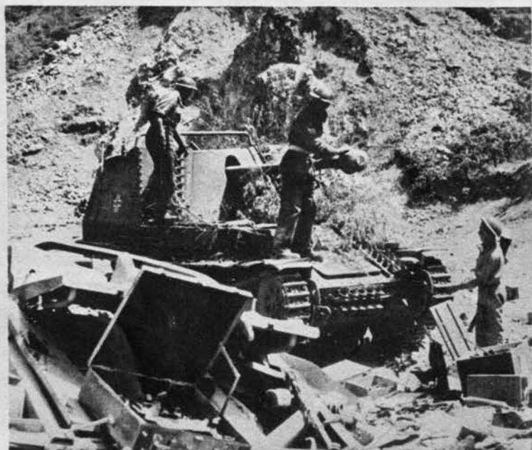
Sloping gun shield of SP "75" projects from gun house. On either side are pieces of track. Rod on the gun house is for crew's support.
